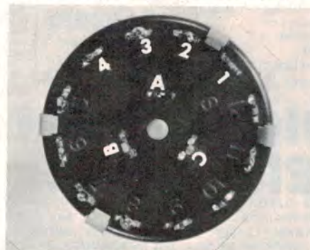
Rear view of a C&K four-position switch showing the connections for SW2.
