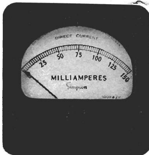
In the photo at the left, the meter is shown before refacing it for the example explained in the text. The "after" view (right) shows the same meter refaced to a 0-150 mA current range.
