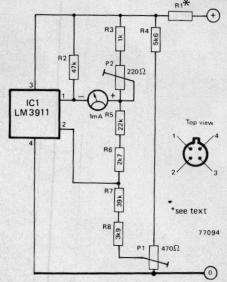
supply voltage is not critical provided the value of R1 is chosen so that about 3 mA flows through it. The value of R1 is given by
