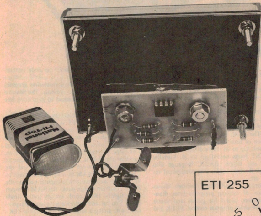
Rear view of the instrument showing general assembly. You may prefer to use a rechargeable NiCad type, rather than the dry battery shown, for battery operation of the unit.
