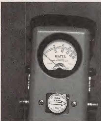
Fig. 9. The Bird Electronics Model 43 RF wattmeter is an old war horse that has served the author well over the years (photo courtesy of Bird Electronics Corporation).
