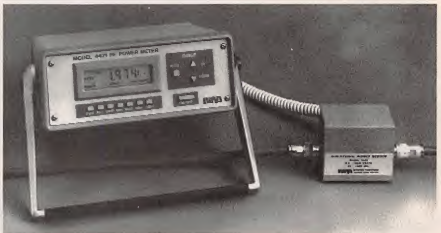
Fig. 10. Bird Electronics Model 4421 RF wattmeter (photo courtesy of Bird Electronics Corporation).
