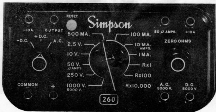
FIG. 3 - 260-5P CONTROL PANEL
