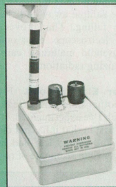
Fig. 4. Charging a dosimeter.
