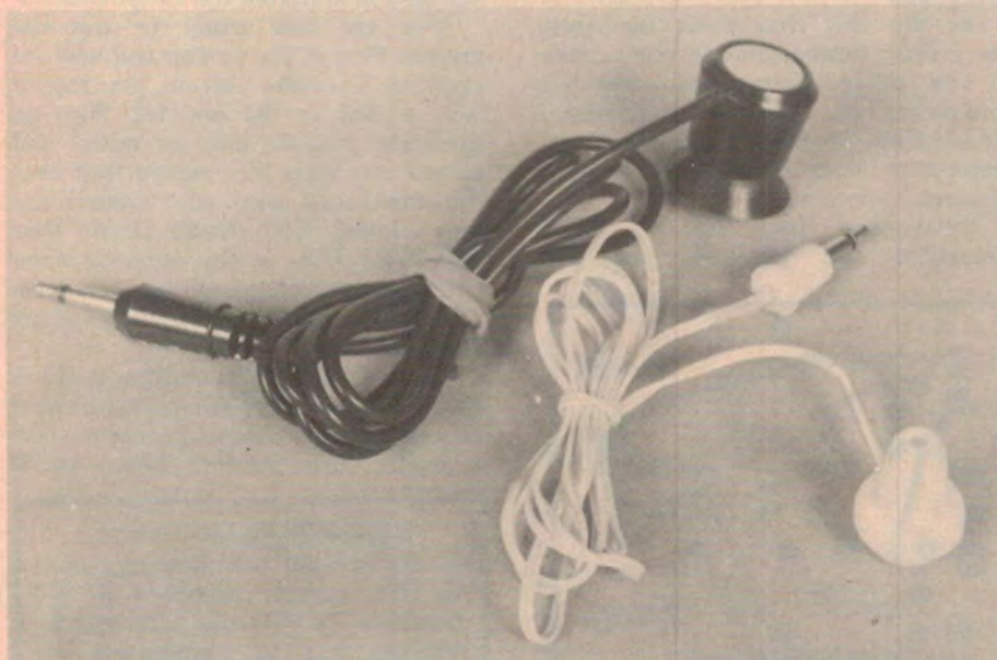
The sensor used for this project is a "telephone pickup coil" — the black object at the top. The inexpensive magnetic earpiece, below the pickup coil, indicates when you have located a cable.
