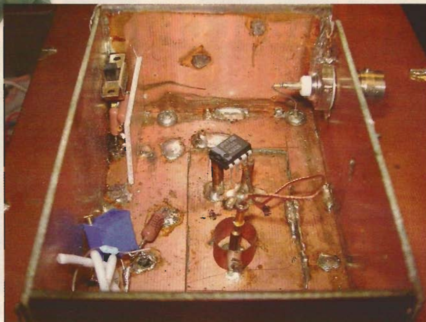
Figure 7 This configuration mounts the DUT on long standoffs that do not touch the PCB. Copper-clad boards serve as shielding (courtesy National Semiconductor).
