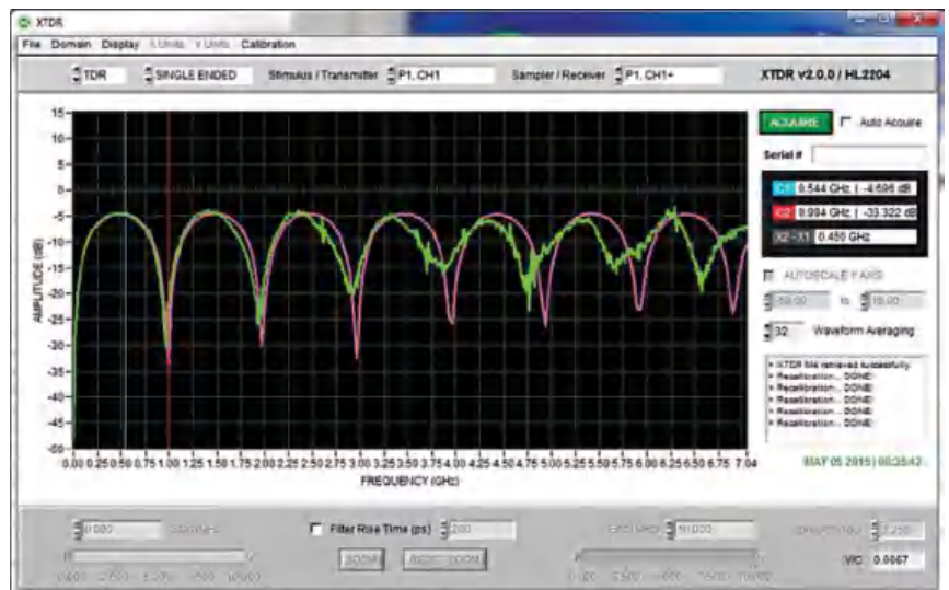
Fig. 7: Comparison of S11 (return loss) measurements taken by XTDR and HL2204 (green trace) versus those taken on a much more expensive VNA instrument (pink trace) (Image courtesy: www.everythingrf.com)
