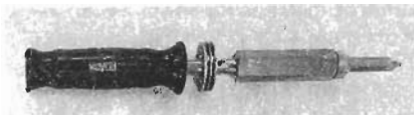
HEAVY-DUTY HEXACON SOLDERING IRON produces 300 watts to heat large areas for soldering.
