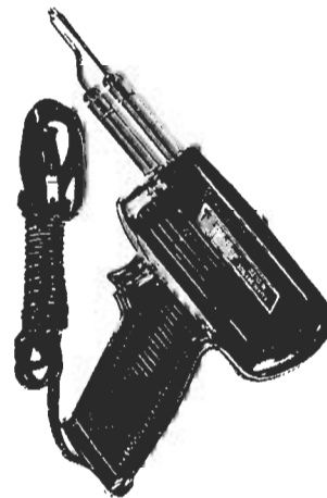
WELLER SOLDERING GUN is still popular for many soldering chores; current heats wire tip.
