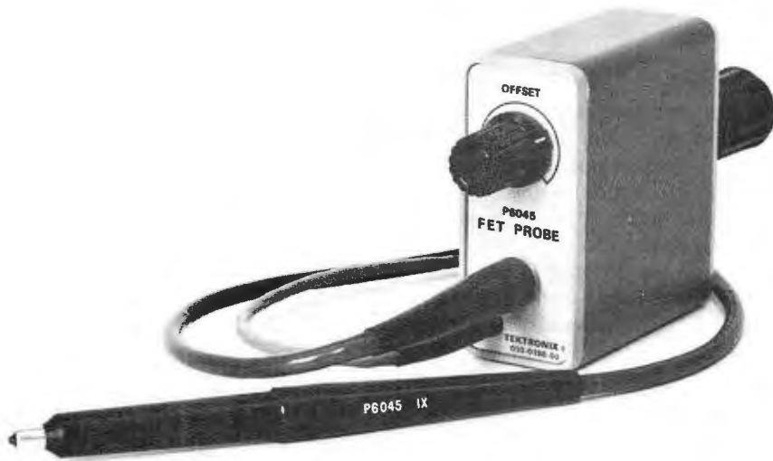
The Tektronix P6045 probe, with FET isolation stage, provides signal attenuation of 1:1, 10:1, or 100:1 with 1.5-ns rise time.
