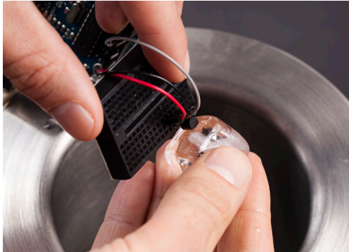
Figure 3-19. Testing the LM35 with an ice cube
