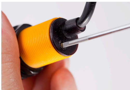
Figure 3-8. Adjusting the infrared sensor
