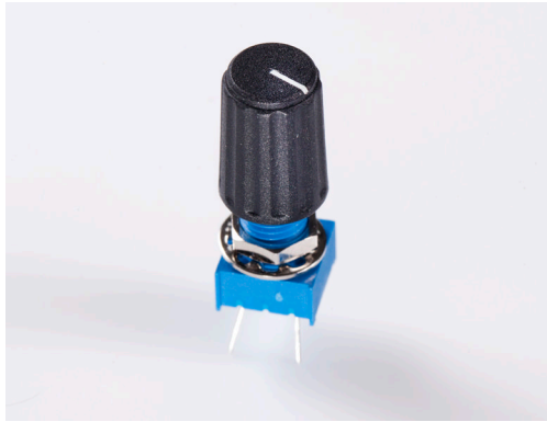
Figure 3-10. Potentiometers can measure rotation
