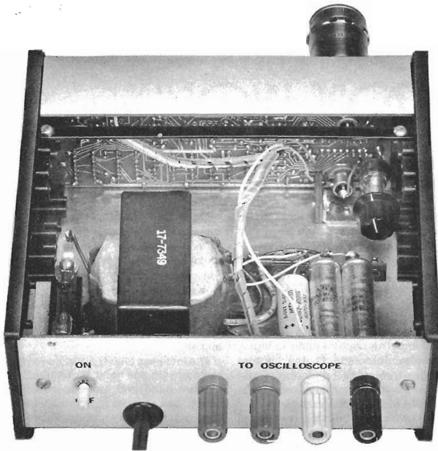
Jacks for scope connections and on/off switch are on chassis rear.
