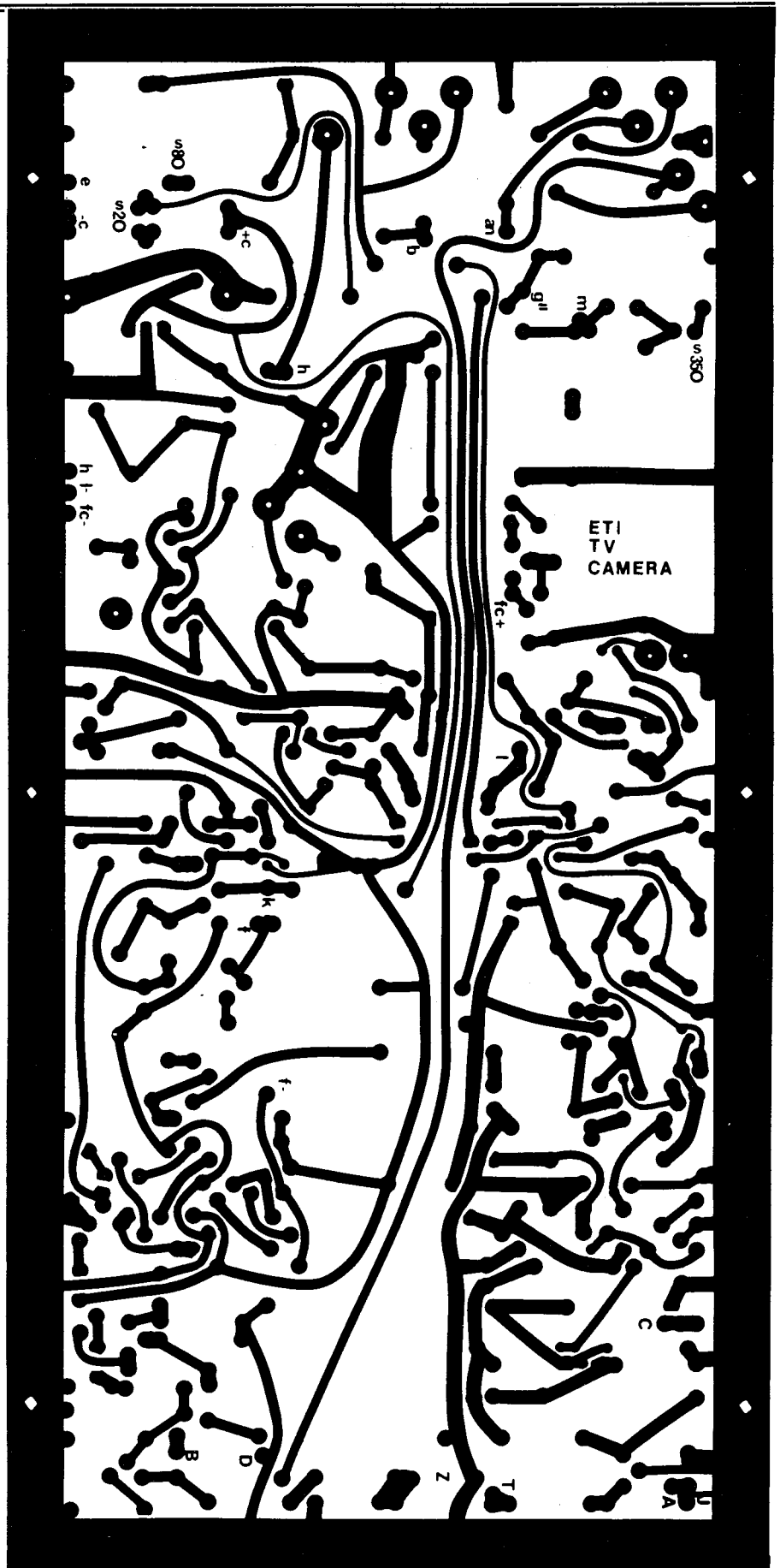
Fig. 7. Full size foil pattern for CCTV camera. Note copyright design is held by Crofton and ETI.
