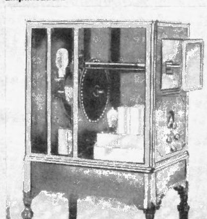
JENKINS PROJECTION RADIOVISOR, developed in 1931, used deForest's new neon-crater tube and a 1-inch scanning disc with sixty 1/2-inch lenses to throw a flying-spot image on the rear of the ground-glass viewing screen.
