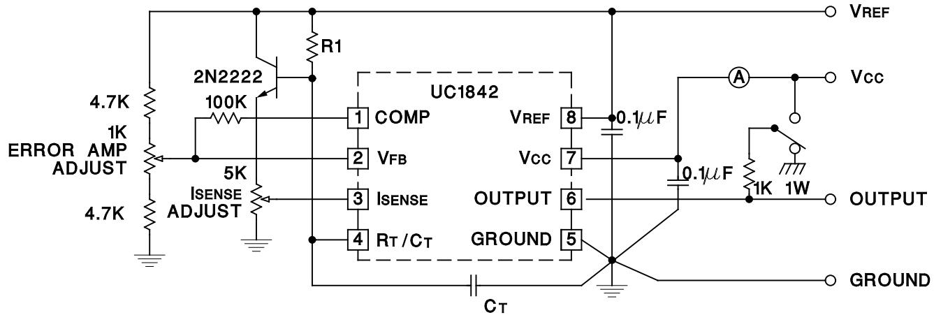
High peak currents associated with capacitive loads necessitate careful grounding techniques. Timing and bypass capacitors should be connected close to pin 5 in a single point
