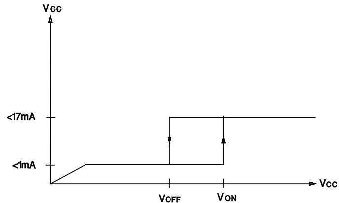
During under-voltage lock-out, the output driver is biased to ground with a bleeder resistor to prevent activating the power switch with extraneous leakage currents.
