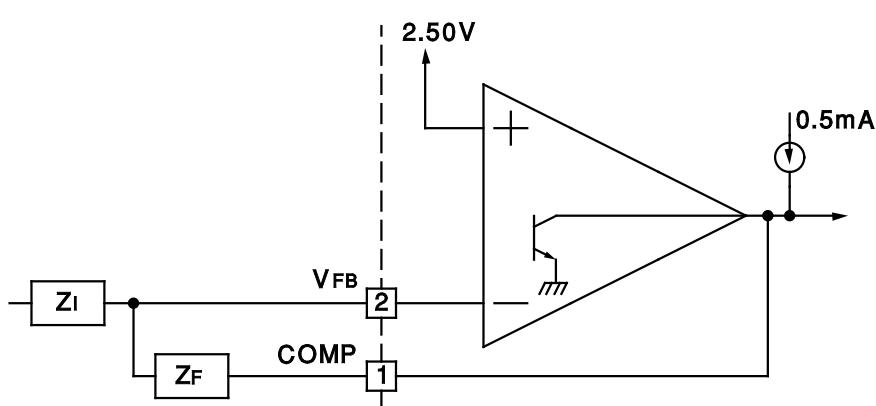
Error Amp can Source or Sink up to  $0.5\text{mA}$
