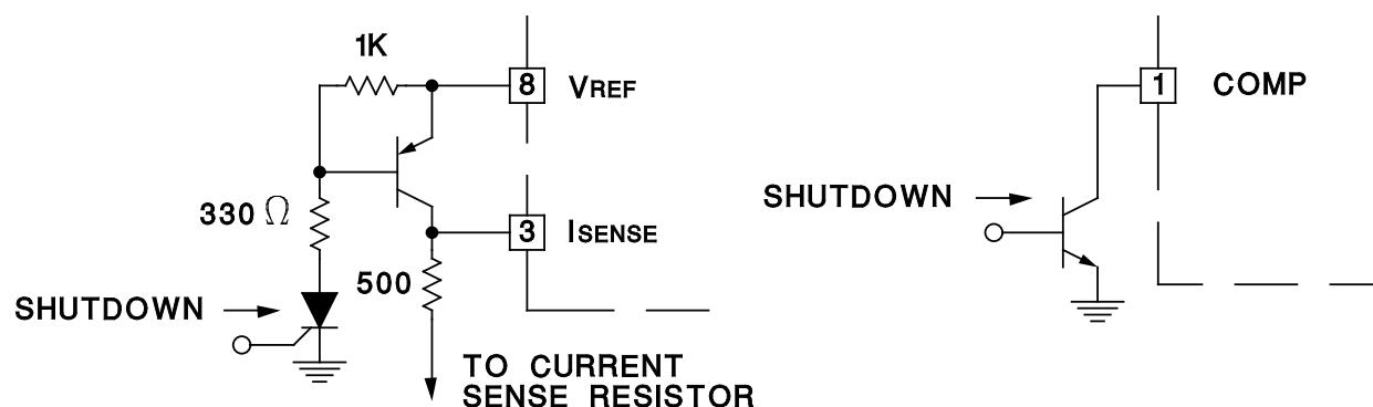
Shutdown of the UC1842 can be accomplished by two methods; either raise pin 3 above 1V or pull pin 1 below a voltage two diode drops above ground. Either method causes the output of the PWM comparator to be high (refer to block diagram). The PWM latch is reset dominant so that the output will remain low until the next clock cycle after the shutdown condition at
