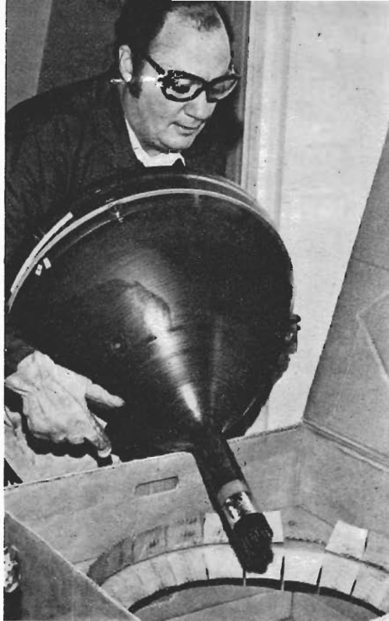
Band is attached to new tube. Be careful to see that the hole in the band is between glass ridges. The ridges indicate the top of the round tube.
