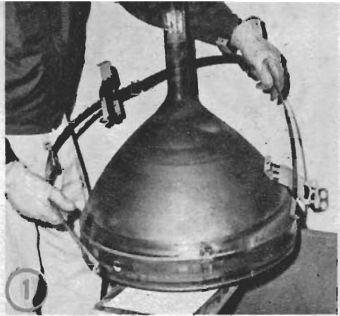
Band is attached to new tube. Be careful to see that the hole in the band is between glass ridges. The ridges indicate the top of the round tube.
