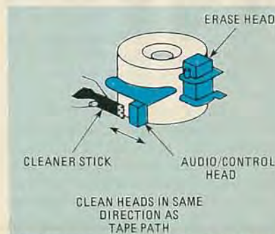
FIG. 21—WHEN CLEANING the audio/control and erase heads, move the cleaning stick horizontally as shown.
