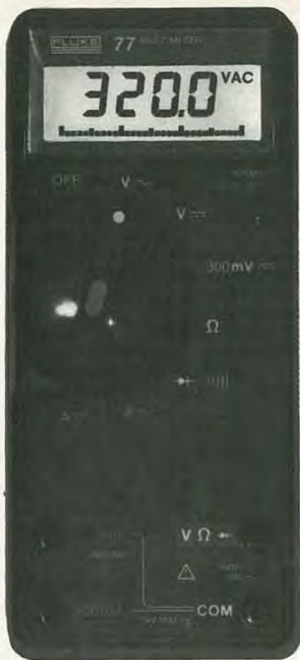
A HANDHELD MULTIMETER like this one should be fine for VCR servicing.
