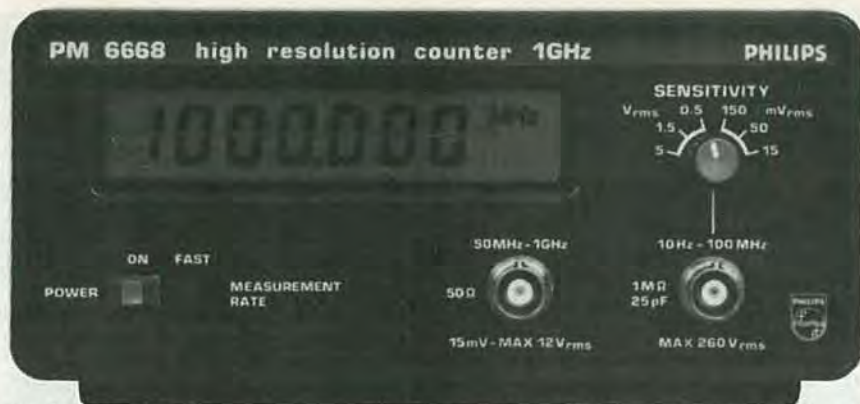
THIS FREQUENCY COUNTER measures frequencies up to 1 GHz. But more important for VCR work, it measures signals down to 10 Hz.
