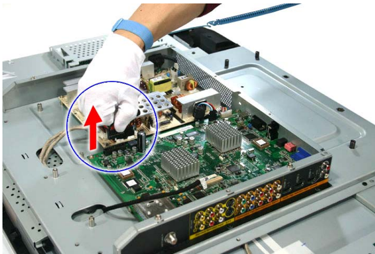
Power jumper (above)
