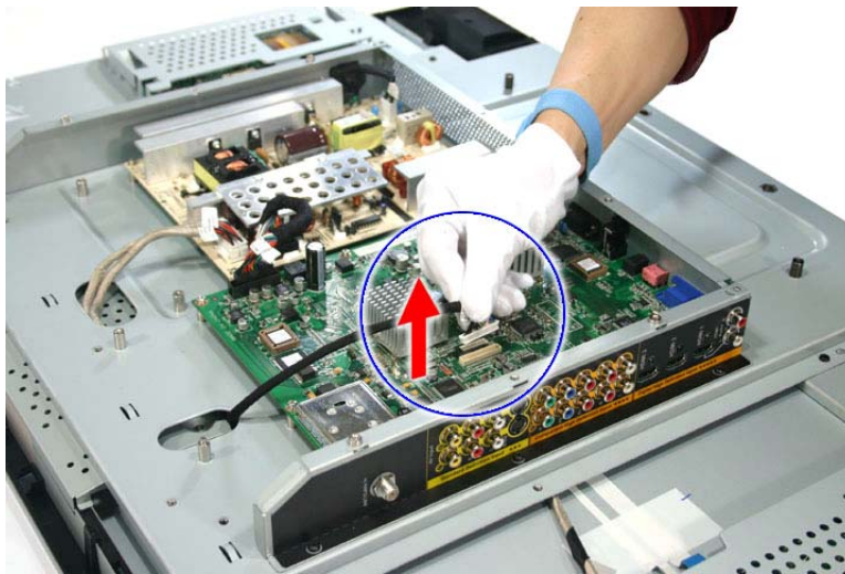
LVDS cable, requires screw removal (above)
