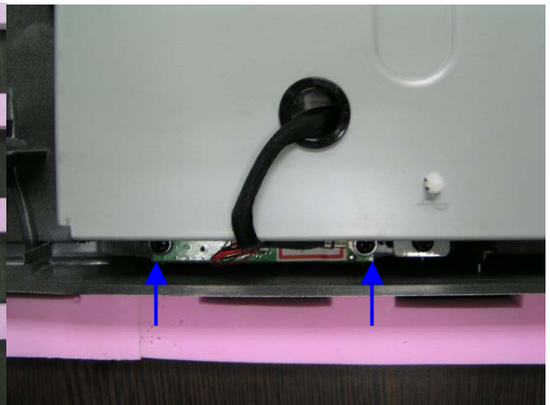
27. Loosen 2 screws on IR board.
