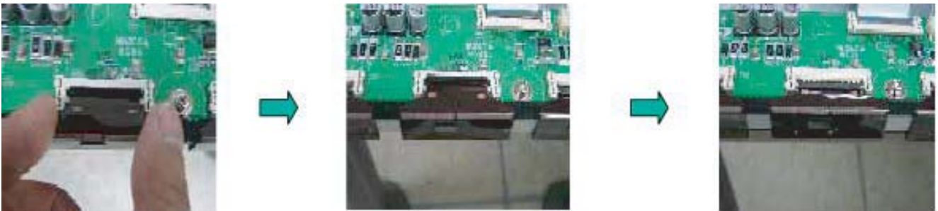
Figure 4-6 Re-assembly of TCP
