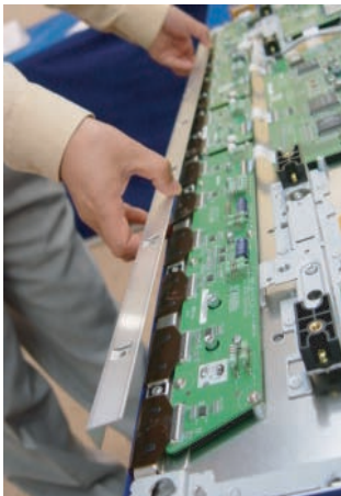
Figure 4-11 Photo 3 - Heat sink removal
