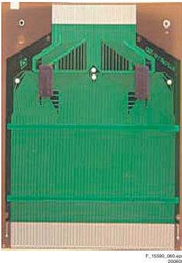
Figure 9-12 Tape Carrier Package
