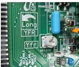
Figure 8-29 Adjusting waveforms - 50" HD W2 & 50 HD W2 Plus [1/2]
