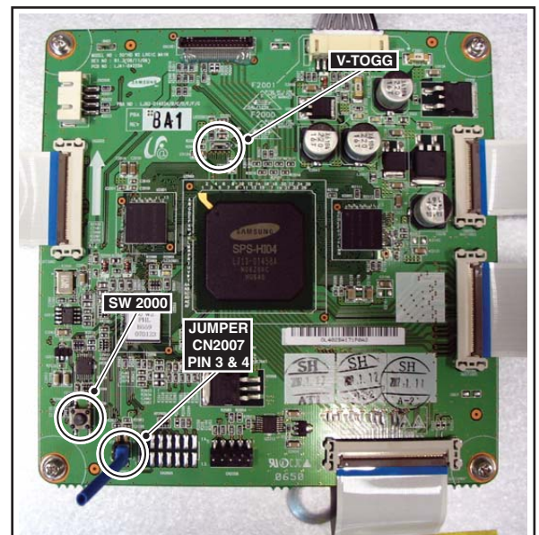
Figure 8-28 Logic PWB - 50" HD W2
