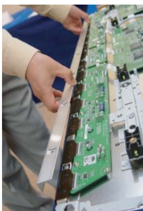
Figure 4-20 Photo 3 - Heat sink removal
