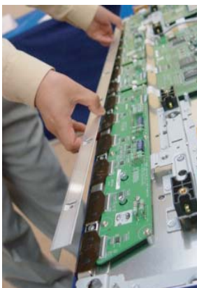
Figure 4-17 Photo 3 - Heat sink removal
