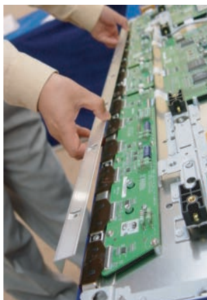
Figure 4-14 Photo 3 - Heat sink removal
