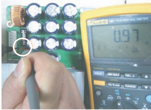
Ve fuse (F4005) – OK (0.x ~ x.x ohm)
