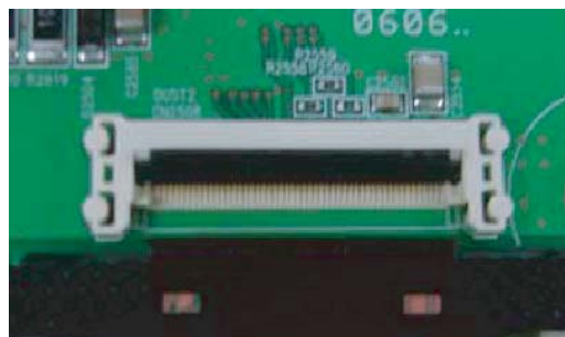
Figure 4-7 Mis-assembly of TCP
