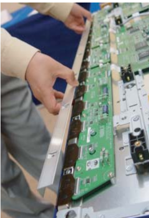
Figure 4-11 Photo 3 - Heat sink removal
