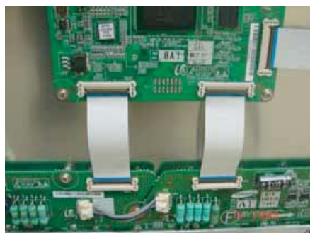
Figure 4-8 Dis- and re-assembly of FFC
