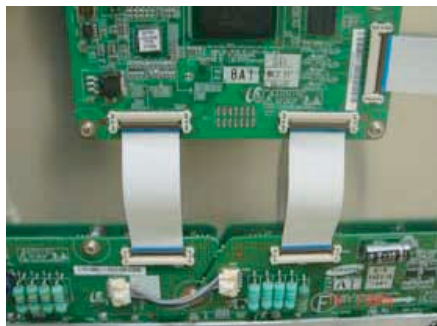
Figure 4-8 Dis- and re-assembly of FFC
