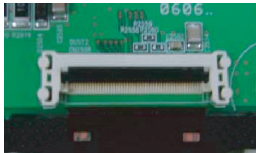
Figure 4-7 Mis-assembly of TCP
