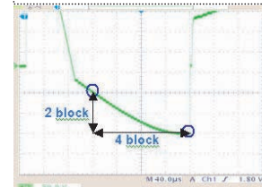
VR5002 Adjustment : Falling Ramp Oscilloscope Setting : 50V / 40us
