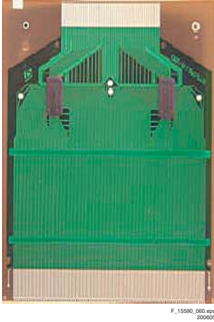
Figure 9-13 Tape Carrier Package
