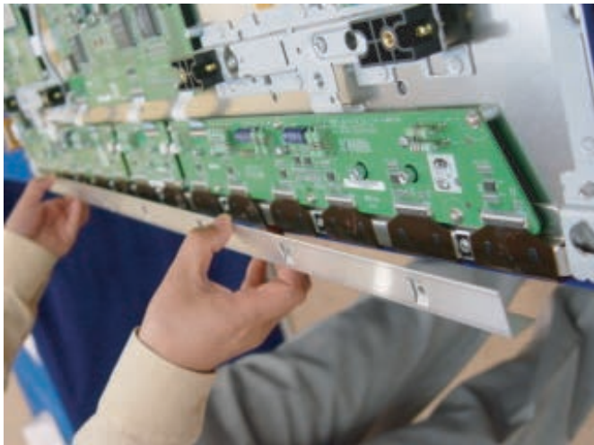
Figure 4-9 Photo 1 - Heatsink removal
