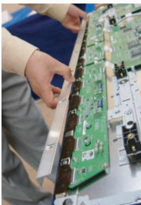
Figure 4-17 Photo 3 - Heat sink removal
