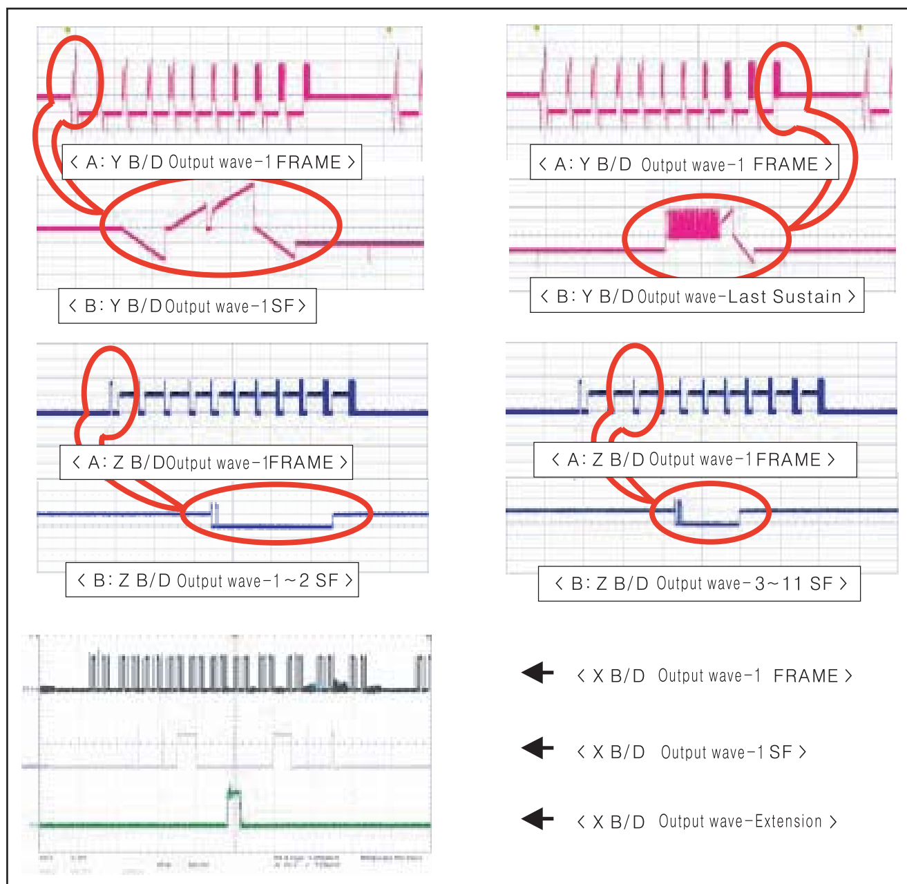
Figure 5-23 Output waveforms on X, Y, and Z-boards
