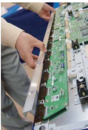
Figure 4-14 Photo 3 - Heat sink removal
