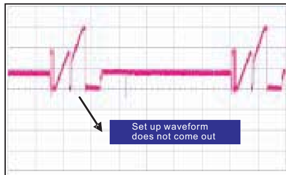
Figure 5-37 Set down FET defective
