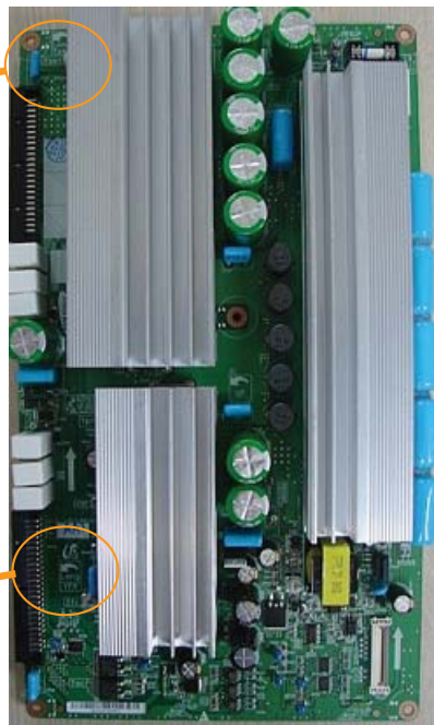
Figure 8-29 Adjusting waveforms - 50" HD W2 & 50 HD W2 Plus [1/2]
